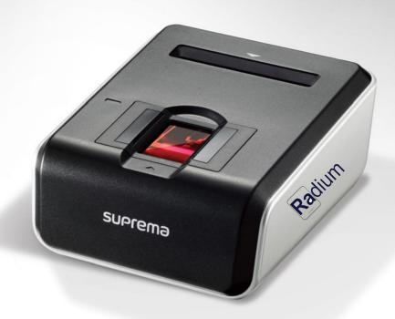
**BioMini Combo** I BioMini Combo has specially been designed to provide a high level dual-authentication security solution for PC based identity access management solutions. Housing with contact smart card reader, BioMini Combo provides the latest 500dpi slim optical sensor, which boasts a large platen size for easy and reliable fingerprints capturing as well as Suprema's advanced LFD (Live Finger Detection) technology.
