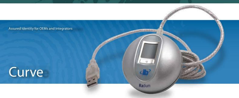
The Curve embodies the future of Fingerprint Biometrics – LES Film imaging technology. Utilizing the same LES Film certified in the world's first non-optical FBI Certified scanner, the Curve establishes the new standard in biometric performance for commercial applications.
