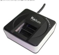
Finger scanning window size: 29 x 29.5mm Scanning area: 25.4 x 25.4 mm (1"x1") Image resolution is 500 x 500 pixels, 500 DPI Color depth 8 bits gray scale No interpolation used Raw fingerprint image file size is 250K bytes USB2.0 high speed only Unique serial number programmed to USB Device Descriptor With a 2M standard USB cable Small size : 75 x 73 x 36 mm
