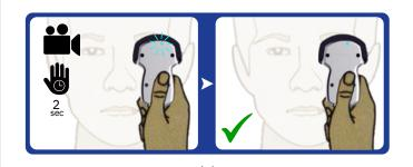
A blinking Blue light indicates the capturing is under process. Wait until the light turn green.
