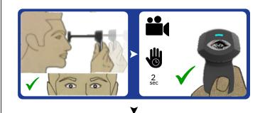
Place the Guide Distance on your eye Capturing occur when blue light blinks. Wait for 2 secs for process to get over.
